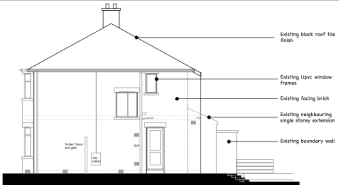
EXISTING SIDE ELEVATION
